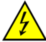
Figure 1 Marking of high voltage equipment
